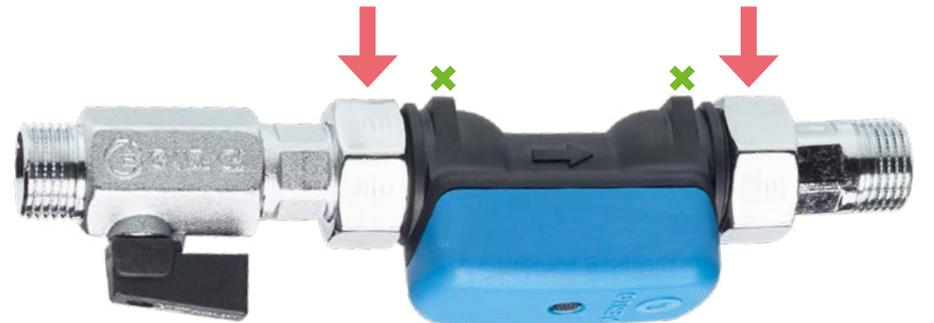
**Note that the body may only be seized with a tool at the place marked with an 'x' (28 mm width of jaw opening).
